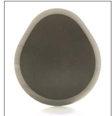
**Fig. 4. Uniformly distributed true contour-hardening patterns produced by CamPro™ machine (courtesy of Inductoheat Inc.)**
