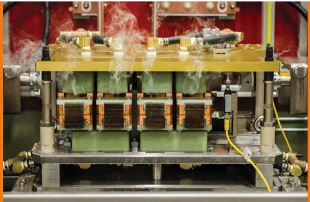
Induction heat treatment is a common method for heat treating different automotive components, including camshafts, which belong to the group of critical engine/powertrain components. Now a new approach makes it possible to induction harden camshafts with almost undetectable distortion.
