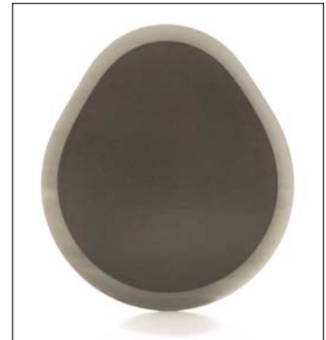
Fig. 4. Uniformly distributed true contour-harden patterns produced by CamPro™ machine (courtesy of Inductoheat Inc.)
